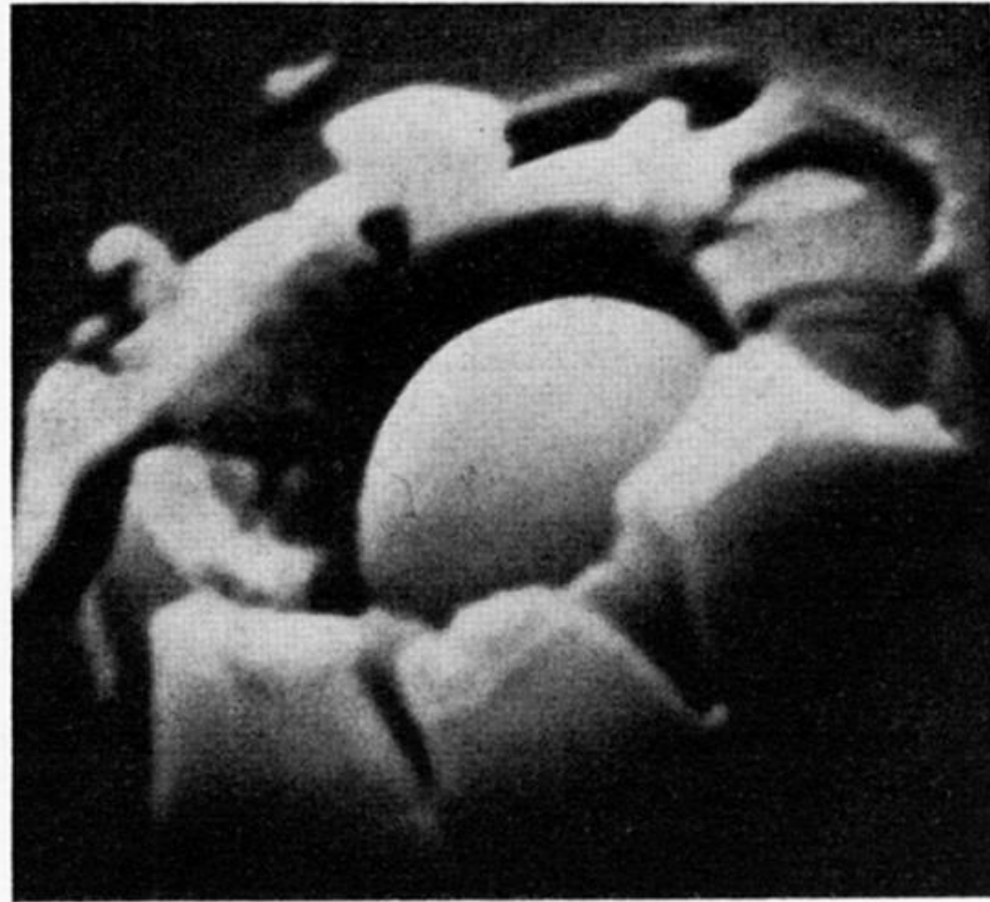
FIGURE 2. During the studies of natural microcraters on light-brown glasses in the Apollo 15 sample 15301,84, a projectile sitting in its crater was observed. (Similar events have been found in simulation experiments with iron microprojectiles.) A microprobe analysis has shown that the natural projectile is mainly composed of iron; the absence of tracks under the crater points to its recent arrival on the Moon.
